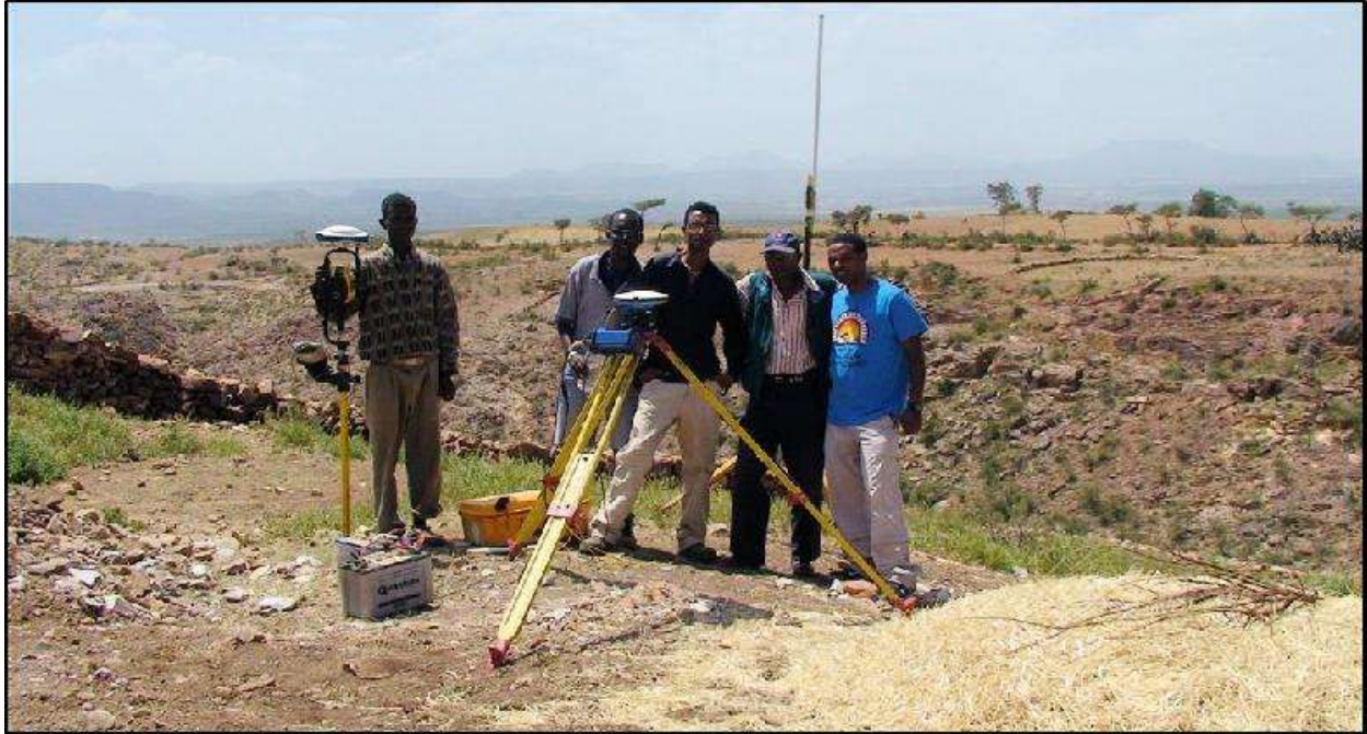
Figure 1. Asmara Project, Eritrea. MWH Geo-Surveys differential GPS survey crew and equipment. Over 45,000 gravity stations were surveyed from 2004 through 2008 using differential GPS instruments from Magellan. All the GPS positions were surveyed in RTK mode with accuracies of 2 cm or better. The Magellan RTK GPS base with a ProMark TM 500 GPS rover are shown in this photo.
